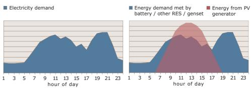
Hybrid systems with a backup genset run with minimal fuel consumption because the genset is brought on line only to assist in periods of high loads or low renewable power availability. This results in a large reduction in fuel consumption as compared to a genset only powered system.
