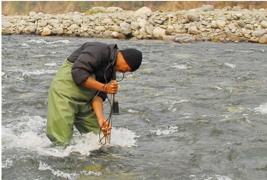
FIGURE 8-6 MEASUREMENT OF DEPTH WITH A WADING ROD
