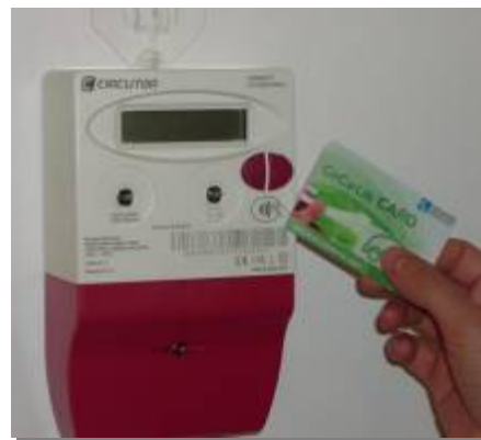
Figure 3: Energy Dispenser Meter (Source: TTA)
