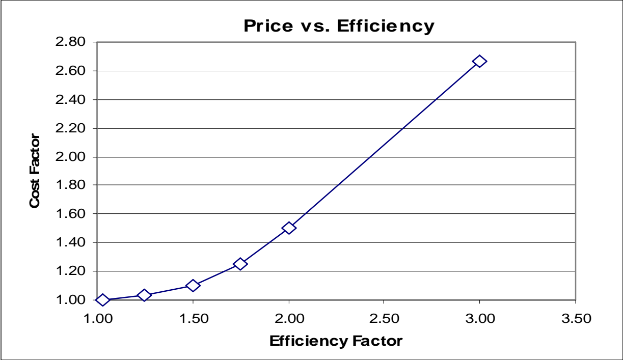
Figure 5.2: Price vs. Efficiency Curve used for Benefit/Cost Analysis* *The cost factor is the price of the average standard-compliant refrigerator divided by the average price of the baseline refrigerator. The efficiency factor is the ratio of the standard-compliant efficiency divided by the baseline efficiency.
